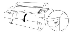
**5** Feed the posterboard into the paper slot until it meets resistance.
