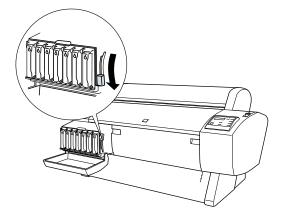
7 If you're using 110 ml cartridges, close the ink compartment cover. If you're using 220 ml cartridges, you'll have to leave the cover open.
