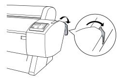
**4** Open the front cover. (The cover has special tabs that act as paper supports when the cover is open.)
