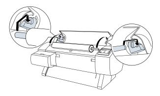
6 Make sure the printer is turned on, then press the Paper Source button until the Roll Auto Cut light comes on.
