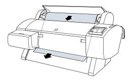
**9** Turn the roll back to remove any slack. Then align the bottom edge of the paper with the row of holes, as shown.
