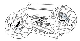
**5** Carefully remove the cutter blade, being careful not to let the spring fly out.
