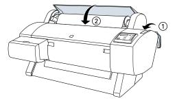
11 Press the Pause button. The paper feeds into the printing position automatically and READY appears on the control panel.
