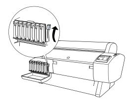
**3** Remove the empty ink cartridge from the printer.
