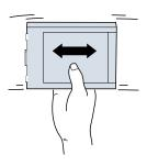
**5** Hold the cartridge with the arrow mark pointing toward the printer. Then insert the cartridge into the slot. Don't force it.
