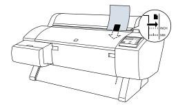
For a large sheet of paper, feed it so that it comes out below. Then align the edges of the sheet with the rows of holes as shown.
