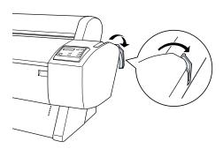
**4** Feed the sheet into the paper slot. Make sure the right edge of the paper is straight and aligned with the scale on the roll paper cover.
